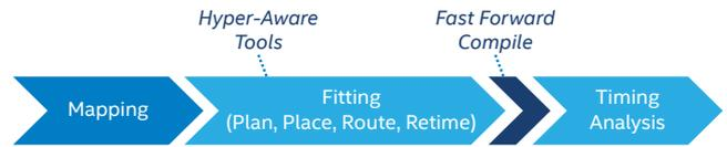
Figure 2. Intel HyperFlex FPGA Architecture Design Flow
