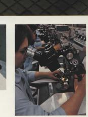
Individual circuits on these wafers are tested by probing and exercising them with a high speed, computer-controlled test system that may conduct a million or more tests in a few seconds. The faulty units are marked for discard when the individual circuits are cut apart.
