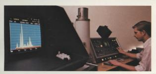
The packaged circuits are returned from Asia to our Santa Clara plant for testing. Here, in rooms with critical temperature control, more extensive electrical tests are performed to assure not only that each circuit performs the desired functions, but that all the electrical parameters are met. At this time, as well as throughout the process, many quality checks are completed and regular samples are taken for extended reliability testing.
